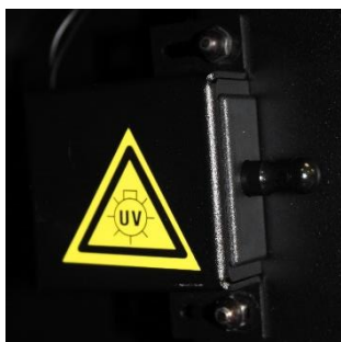
UV Safety Switch
